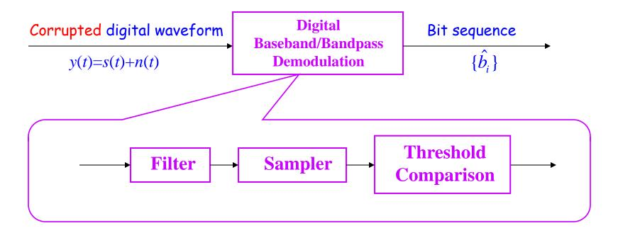
How to design the filter, sampler and threshold to minimize the BER?
