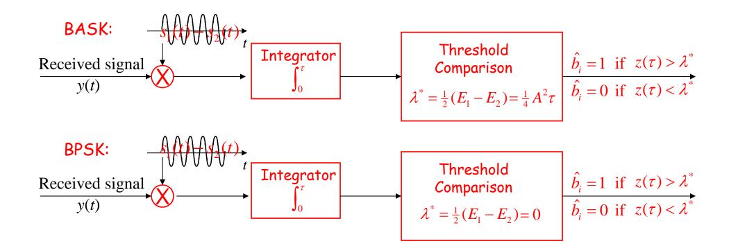
The optimal receiver is also called "coherent receiver" because it must be capable of internally producing a reference signal which is in exact phase and frequency synchronization with the carrier signal  $\cos(2\pi f_c t)$ .
