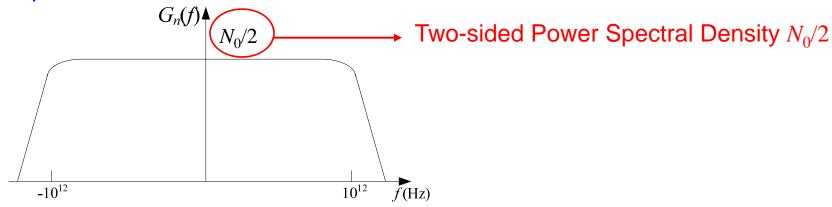
The thermal noise is also referred to as additive white Gaussian Noise (AWGN), because it is modeled as a white Gaussian WSS process which is added to the signal.
